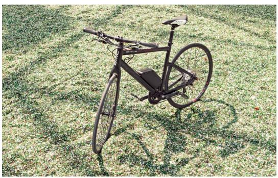
Maxon Bikedrive. With its micromotors, drive specialist Maxon of Sachseln has made the life of NASA astronauts easier. And with the hub motor, Bikedrive has turned a bicycle into an e-bike. With the new motor it can now shoot off like a rocket – from 0 to 30 kilometers per hour in 3 seconds!
